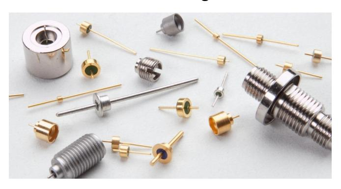
Century Seals manufactures a variety of single pin feed-through terminals. Typical designs include 50 ohm and DC terminals. SMP connectors and custom designs are also produced. Materials include Kovar, CRS, Stainless Steel, and #52 Alloy. Plating types include High Purity Gold, Tin/Lead, Electrolytic and Electro-less Nickel. Contact us for a quote for your specific needs.
