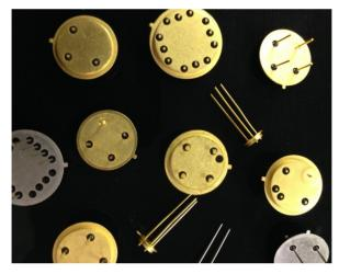
Century Seals manufactures a variety of TO style packages for use in sensor applications. Typical designs include .500 and .600 diameter TO-8, TO-5, and TO-46 headers. Additional custom designs are also produced. Multiple pin configuration styles are available including; ground pins, nail head, straight and custom formed leads. Plating types include High Purity Gold, Electrolytic and Electro-less Nickel. Contact us for a quote for your specific needs.
