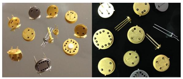
Century Seals manufactures a variety of TO style packages for use in sensor applications. Typical designs include .500 and .600 diameter TO-8, TO-5, and TO-46 headers. Additional custom designs are also produced. Multiple pin configuration styles are available including; ground pins, nail head, straight and custom formed leads. Plating types include High Purity Gold, Electrolytic and Electro-less Nickel. Contact us for a quote for your specific needs.
